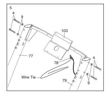
6. Set the Console Cover (87) on the Uprights (77, 79). Make sure that the Console Cover is oriented with the ties toward the bottom as shown.
